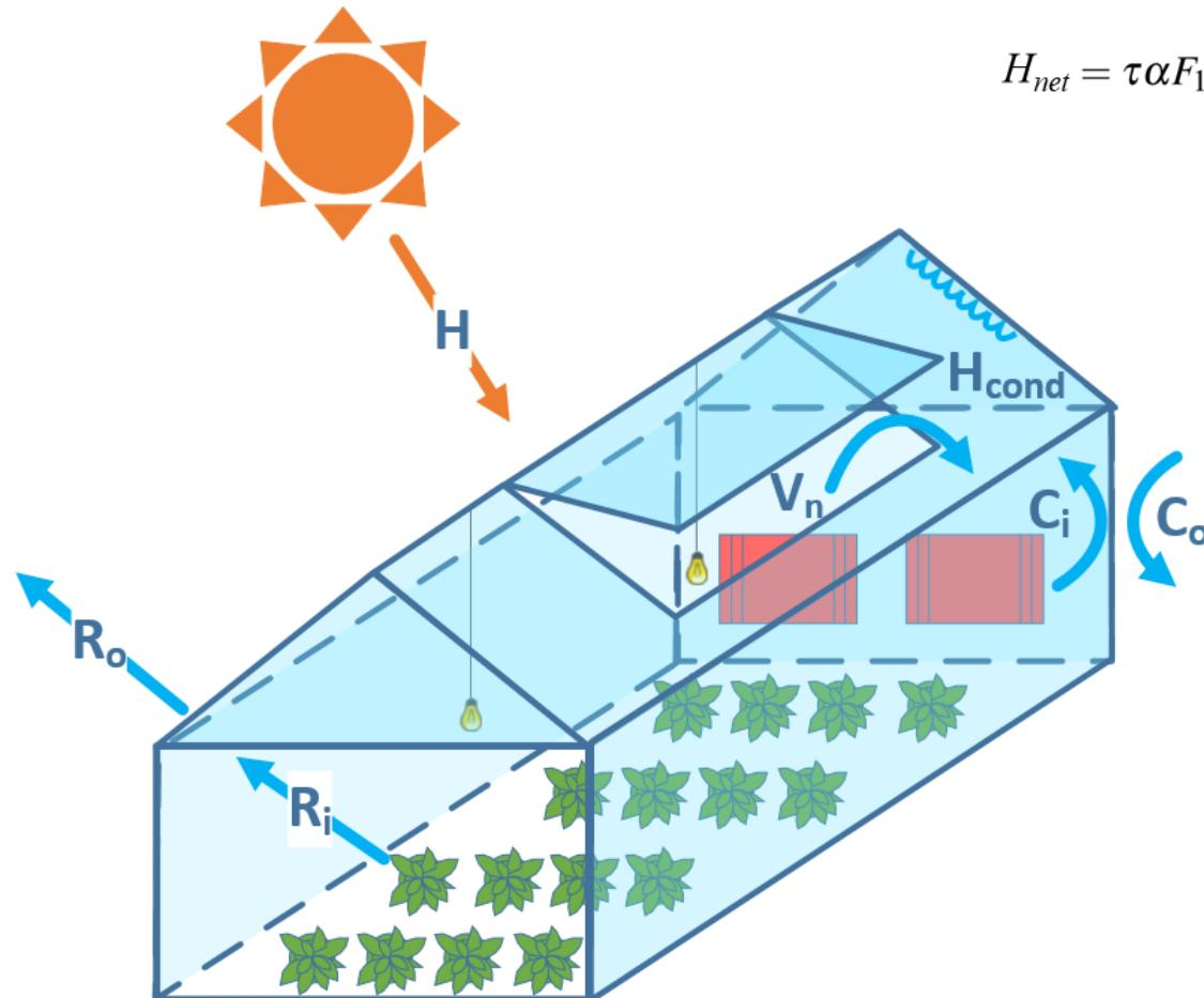
$$H_{net} = \tau\alpha F_1 F_2 A_f H(t) - U(t)A_c(T_{ai}(t) - T_{ao}(t))$$
